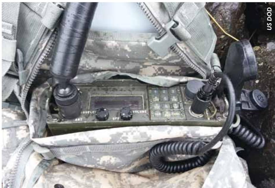
**The US Army's AN/PRC-155 manpack radio is one of several transceivers which has received the MUOS waveform which will help troops to communicate in jungles. It is one of several transceivers to have received this new waveform.**
