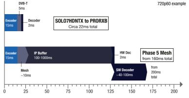
Typical End-to-End Delay/ms
