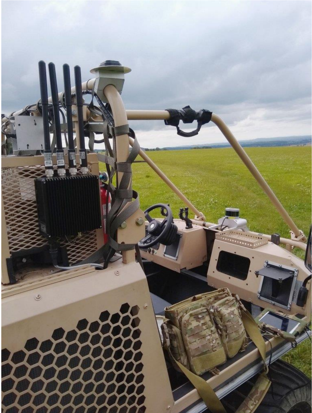
The Domo Tactical Communications NETNode2x5W-5RM MANET radio mounted on a Hippo unmanned ground vehicle during British Army trials. (Domo Tactical Communications)
