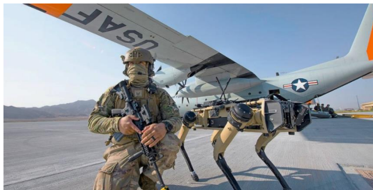
A Silvus Technologies StreamCaster radio mounted on a Ghost Robotics V60 legged unmanned ground vehicle during a USAF ABMS Onramp Experiment. (Silvus Technologies)
