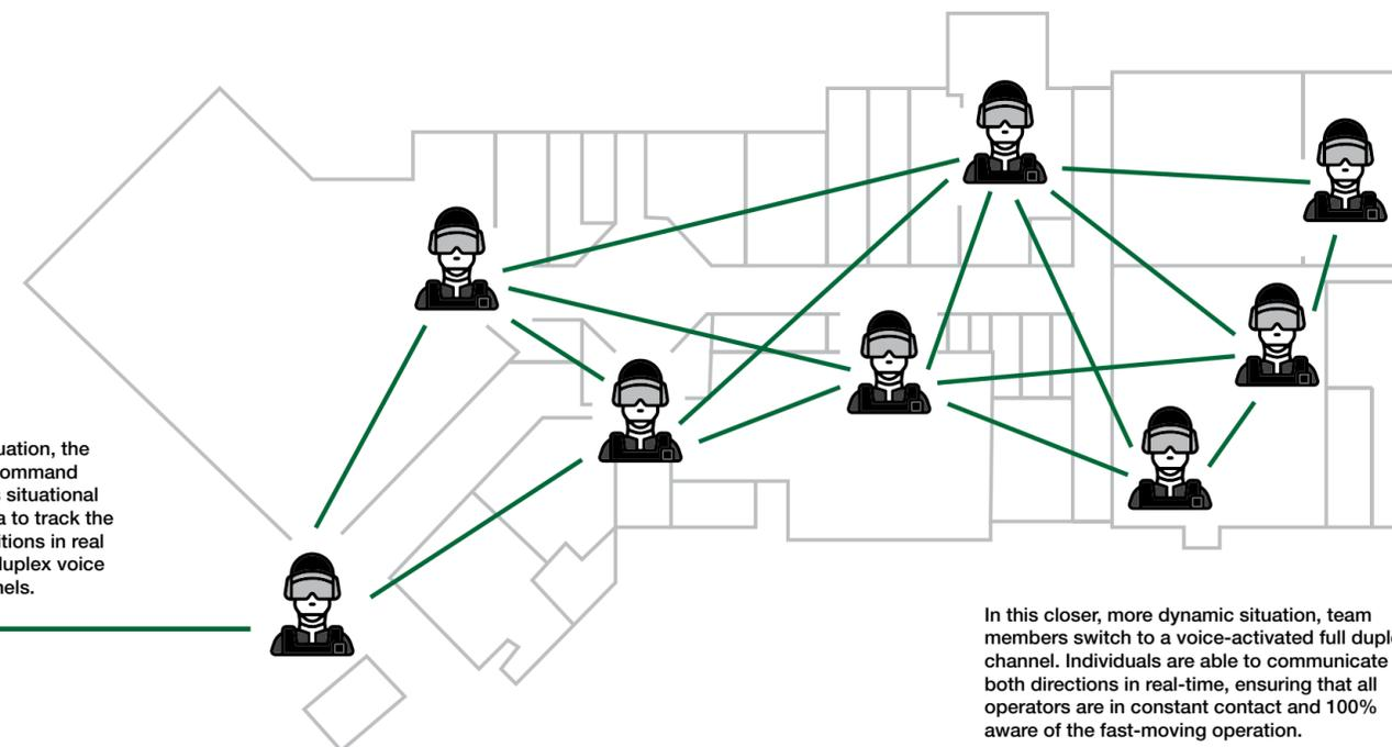
In this closer, more dynamic situation, team members switch to a voice-activated full duplex channel. Individuals are able to communicate in both directions in real-time, ensuring that all operators are in constant contact and 100% aware of the fast-moving operation.
