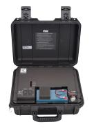
Codan's ET-5 provides the smallest footprint of any transportable P25 repeater supporting transparent encryption in VHF/UHF, or 800 MHz bands. It operates with standard alkaline D-Cell batteries available everywhere, or a rechargeable lead acid battery.
