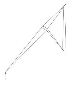
The Semi-Delta Antenna is an economical broadband base station antenna suitable for short to medium distance HF communications. The compact design of the antenna makes it suitable for installations that have limited space available.
