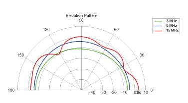
Note: Antenna radiation patterns are based on perfect earth conditions. Azimuth plots are at 35° elevation. Elevation plots are taken broadside from antenna.
