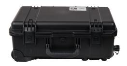
Codan's Stratus Power Center is a 35Ah battery housed in a compact and rugged polypropylene copolymer transportable case for power support of the CODAN Stratus Repeater. The Power Center provides a 12VDC power source that is charged by a 15VDC input from an AC/DC 15VDC power supply or optional solar panel.
