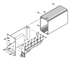
Remove the four front panel screws (A) and four side panel screws (D) to slide the receiver outer cover off and expose the IF / Audio Main Board Local Oscillator and Front End Assemblies. Remove the two front panel screws (B) and internal screw (C) to remove the Front End for easier access to the Local Oscillator.
