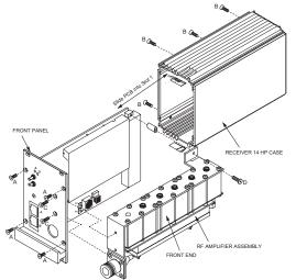
Remove the four front panel screws (A) and four side panel screws (B) to slide the receiver outer cover off and expose the Main Board, Controller and DSP Boards, RF Board and Front End Assemblies. Remove the two front panel screws (C) and internal screw (D) to remove the Front End Assembly.
