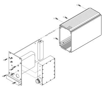
Remove the four front panel screws (A) and four side panel screws (C) to slide the receiver outer cover off and expose the IF / Audio Main Board Local Oscillator and Front End Assemblies. Remove the two front panel screws (B) to remove the Front End.
