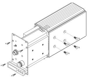
Remove the four front panel screws (A) and four side panel screws (B) to slide the transmitter outer cover off and expose the Main Board, Local Oscillator, Audio Processor Board and Amplifier.
