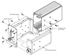
Remove the four front panel screws (A) and four side panel screws (B) to slide the transmitter outer cover off and expose the Main Board, Controller and DSP Boards, RF Board and Amplifier. Remove the two front panel screws (C) and the four internal screws (D) to remove the Amplifier Assembly.
