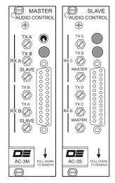
Common modes of operation used in a multi-transceiver system including audio routing, PTT / COR and COR / RX MUTE sequence, hang timer settings, CTCSS and DTMF settings, battery monitor and acknowledge tone, are selected on the master audio control card.
