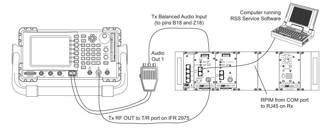
On the IFR 2975, recall Daniels setup 7 (Tx\_Ana) from your internal drive. Enter the correct RF frequency on the IFR 2975, set the MIC MODE switch on the front panel of the transmitter to Analog, and flip the other switch to KEY TX.
