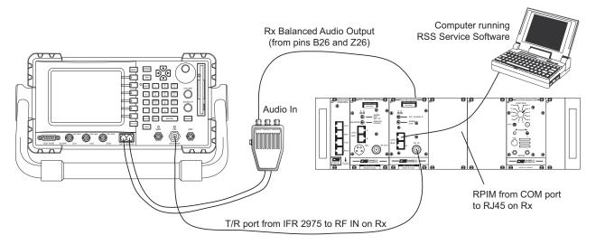
On the IFR 2975, recall Daniels setup 1 (Rx\_Ana) from your internal drive. Enter the correct RF frequency, select the MOD TYPE to FM and set it for a 1.0 KHz tone and ensure that the deviation level is set correctly for your receiver (wide / narrow). Enter the CTCSS tone (if used) and deviation level.
