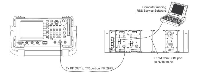
On the IFR 2975, recall Daniels setup 8 (Tx\_CTCSS) from your internal drive. Enter the correct RF frequency on the IFR 2975, set the MIC MODE switch on the front panel of the transmitter to Analog, and flip the other switch to KEY TX.
