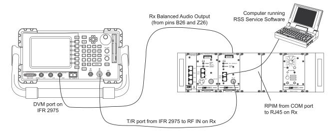
Adjust the Rx Balanced Audio Output level adjustment (R34 on MT-4D, R6 on MT-4R) for -8.0 dBm audio level (308 mVrms @ 600 ohms). The high and low alarms are set at -7.5 dBm and -8.5 dBm audio levels.
