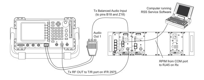
On the IFR 2975, recall Daniels setup 9 (Tx\_Dig) from your internal drive. Enter the correct RF frequency on the IFR 2975, set the MIC MODE switch on the front panel of the transmitter to Digital, and flip the other switch to KEY TX.
