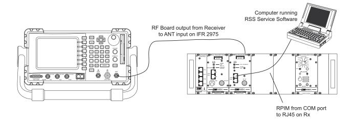
The reference oscillator test on the receiver requires a connection directly into the RF Board, which uses an SMB connector. The SMB-BNC adapter is required for this connection. On the MT-4R equipment, a small SMB-SMB cable is required to connect to the SMB jack that is mounted on the RF Board (beneath the Front End). On the MT-4D equipment the SMB-BNC adapter can be plugged directly into the cable that is normally connected to P2.
