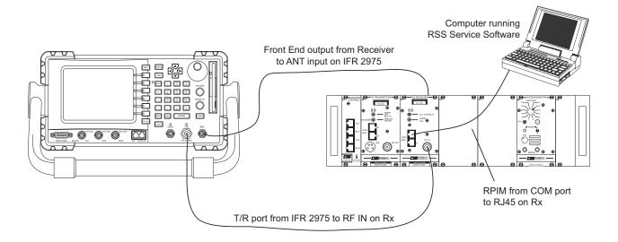
The internal cable in the receiver from the output of the front end terminates in an SMB connector. On the MT-4R equipment the SMB plugs directly into the RF Board. Disconnect the SMB cable from the RF Board connector and use the SMB-BNC adapter to connect this point to the ANT input on the IFR 2975. On the MT-4D equipment the SMB plugs into P6 on the Main Board. Disconnect the SMB cable from the P6 and use the SMB-BNC adapter to connect this point to the ANT input on the IFR 2975.
