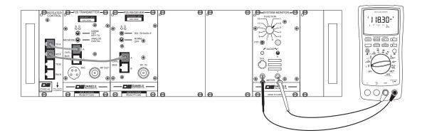
The FUNCTION rotary switch on the front panel of the System Monitor will allow you to test various points in the radio system. Following is a list of System Monitor rotary switch positions, the functions they measure and the parameters measured (please note that switch position 8 requires a carrier and audio tone injected into the receiver):
