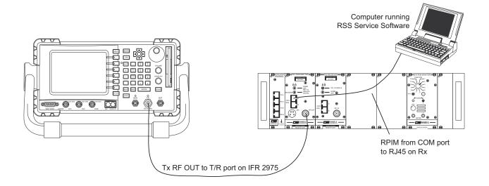
On the IFR 2975, recall Daniels setup 10 (Tx ModFid) from your internal drive. Enter the correct RF frequency on the IFR 2975 and set the transmitter front panel switch to NORM. The MIC MODE switch on the front panel can be set to either Digital or Analog (this test does not make use of the front panel switch).
