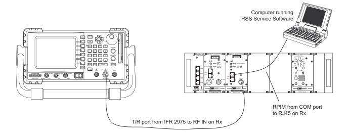
On the IFR 2975, recall Daniels setup 3 (Rx\_BER) from your internal drive. Enter the correct RF frequency, select the MOD TYPE to P25 and set it for the STD 1011 test pattern (the 1011 test pattern will not operate correctly for this test).
