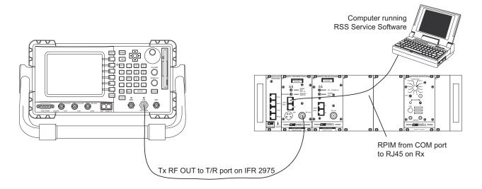
On the IFR 2975, recall Daniels setup 11 (Tx\_VHFRef) or setup 12 (Tx\_UHFRef) from your internal drive. The RF frequency is automatically set for either the VHF or UHF reference frequency (depending on the file recalled). Set the transmitter front panel switch to NORM. The MIC MODE switch on the front panel can be set to either Digital or Analog (this test does not make use of the front panel switch).
