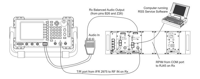
On the IFR 2975, recall Daniels setup 2 (Rx\_Dig) from your internal drive. Enter the correct RF frequency, select the MOD TYPE to P25 and set it for the SPEECH test pattern (or optionally the 1011 test pattern).
